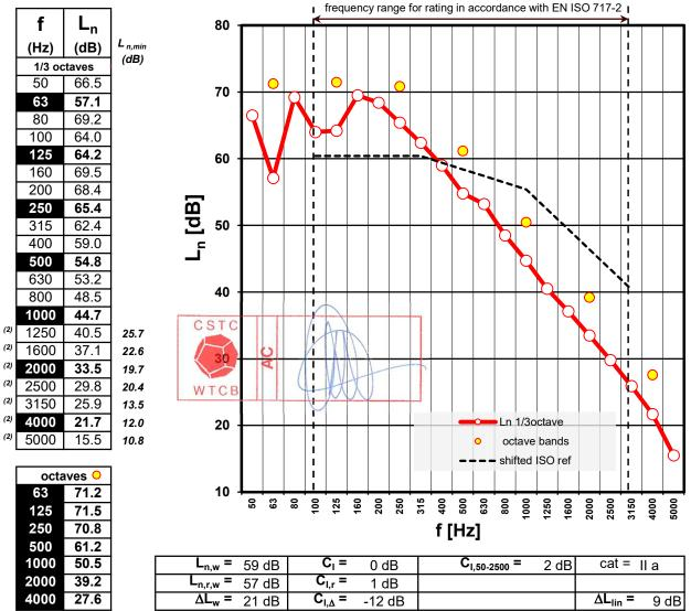
Rating based on laboratory measurement results obtained by an engineering method
